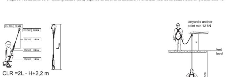
H[m] – distance between lanyard's anchor point and a user's feet
